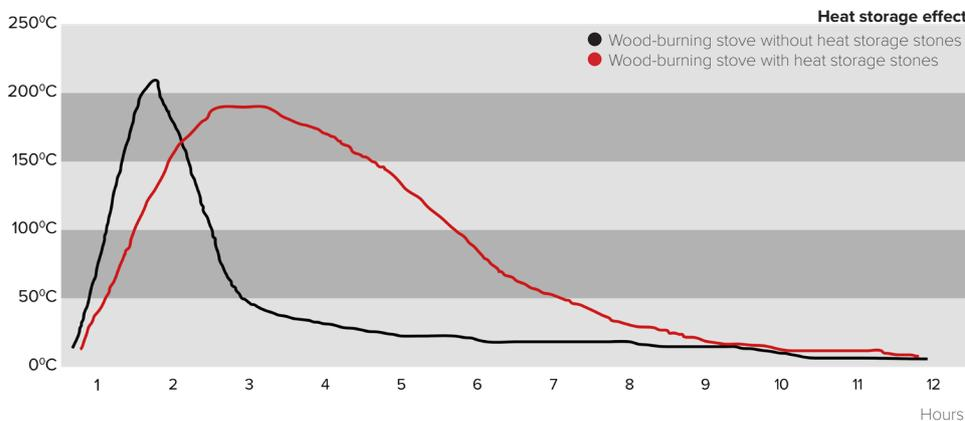
A wood-burning stove with heat storage stones means more continuous heat in the room with the same amount of firewood.
